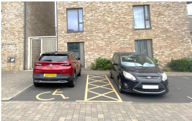
Figure 5-2: Appropriate location of accessible parking bay 32
